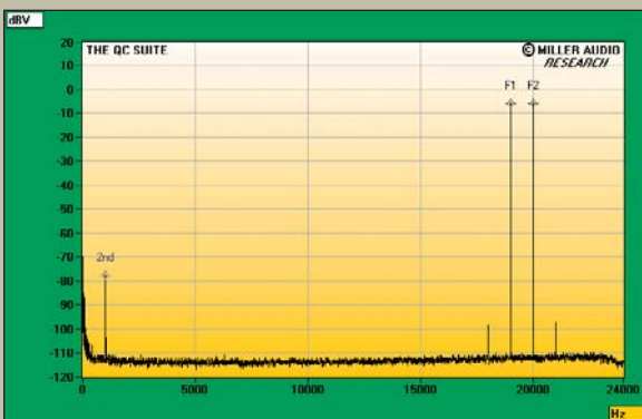
Fig.12 EAR 912, unbalanced HF intermodulation spectrum, DC-24kHz, 19+20kHz at 1V into 8k ohms (linear frequency scale).
