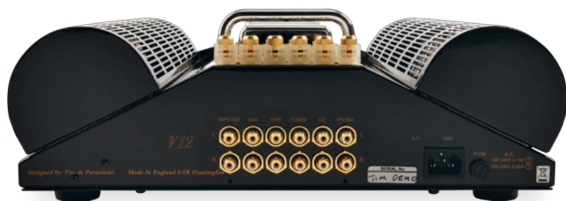
ABOVE: No mysteries here, just IEC mains in, fuse access, RCA sockets for line inputs (phono requires a phono preamp) and vertical sockets for bare wire or banana plugs
