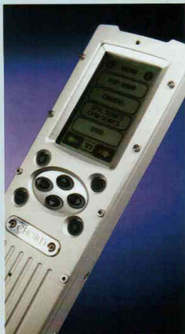
LEFT: The current remote control handset, subject to being replaced shortly, is a learning unit with touchsreen control
